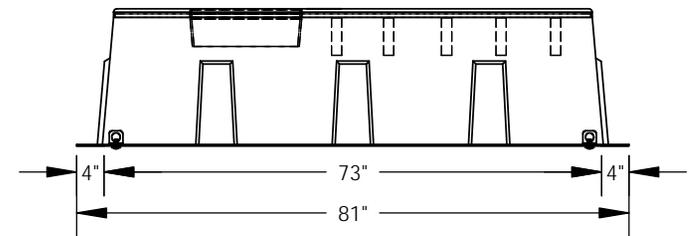
Proper installation of a box pad for transformers over 9,000 lbs. requires the soil to have a compaction level of 98% prior to setting the box pad. If that is not Achievable, a cement pad/footing must be poured underneath the box pad prior to installation.
